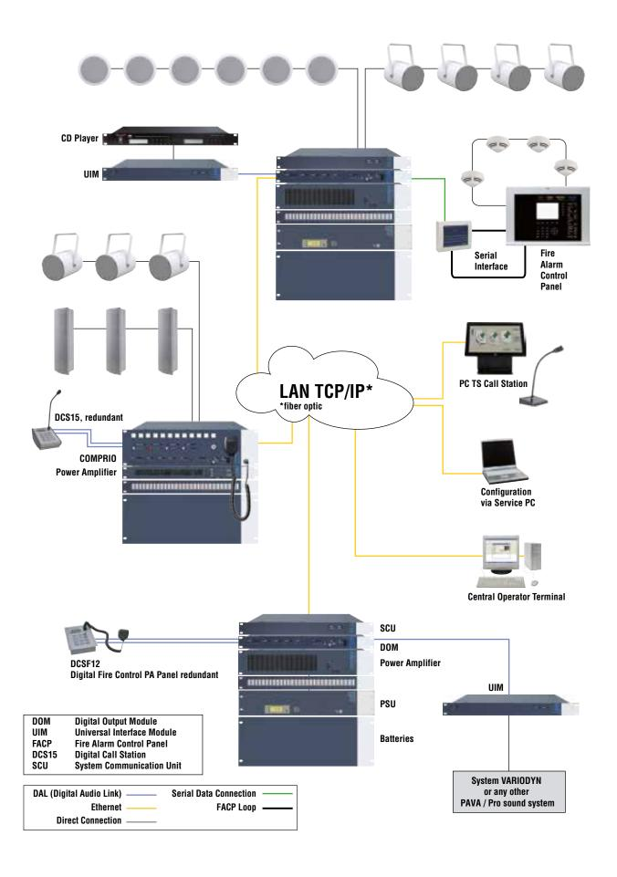
VARIODYN D1 DOM firmware allows to connect up to 400 units and get advantage of the new logical functions, which make it much easier and efficient to configure the DOM. With the firmware comes also the option to connect call stations with a second cable. So it is now possible to do the cable connection to the call station in a redundant way.
