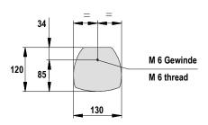
Passive 100 V loudspeaker, with weatherproof aluminium housing, designed for use with voice alarm systems - certified according to EN 54-24, Type B, equipped with two high-quality 4" drivers with treated cones for optimum efficiency in speech and voice alarms.
